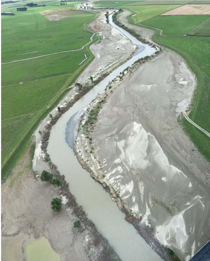
Figure 9: Oroua River downstream of Kopane Bridge showing silt build up after Cyclone Gabrielle. The silt build up will have reduced the flood protection levels provided by the stopbanks.
